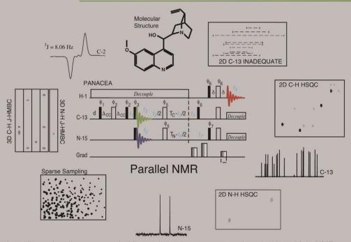
Several spectra of various dimensionality are recorded in parallel using systems equipped with multiple NMR receivers thus increasing the information content of modern NMR experiments. Structure of small molecules can now be determined unambiguously in minutes when parallel NMR is complemented with non-conventional sampling techniques and high sensitivity instrumentation, as described by E. Kupce and R. Freeman in their "Perspectives in Magnetic Resonance" article.
